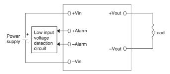
The input voltage detection output terminal ( $\pm$ Alarm) is a transistor output of a photo-coupler and it is insulated at the both input and output sides.
