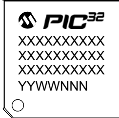
64-Lead QFN (9x9x0.9 mm)
