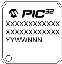
100-Lead TQFP (12x12x1 mm)
