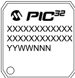
100-Lead TQFP (12x12x1 mm)
