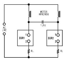
The resistors are unnecessary if the control circuit is designed to ensure that one SSR is off before the other SSR is on.
