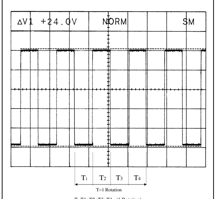
T=T1+T2+T3+T4 = (1 Rotation) $T1=T2=T3=T4= \frac{60}{4 \times \text{rpm}}$
