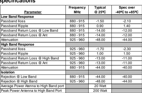
Note: Supplier shall test each filter to the critical electrical specifications of the above table. Any subsequent audits may deviate from in value due to measurement repeatability among different test systems. Power test will be completed with 50 watts average power in 5 MHz steps across the band. 12 steps total with a 100 millisecond pulse at each frequency point and a 200 watt peak, 1% duty factor with a 9 microsecond pulse. Such deviations shall not exceed the following limits:
