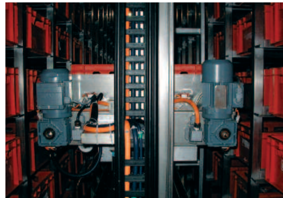
Control cable chainflex® CF10 in storage and retrieval units for high-bay warehouses. e-chain®: System E2 medium
