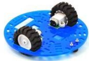
Note: This bracket also works with the 1000:1 micro metal gearmotors, but because of its longer gearbox, it does not fully enclose the exposed gears the way it does on the other micro metal gearmotors. This bracket does not work with our quadrature encoder when used with the 1000:1 micro metal gearmotor.
