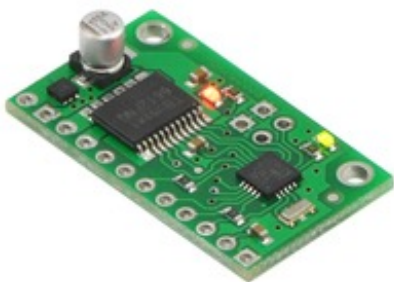
Pololu qik 2s9v1 dual serial motor controller.
