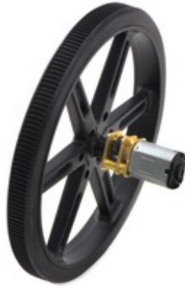
Black Pololu 90×10mm wheel on a Pololu micro metal gearmotor.
