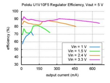
The maximum achievable output current is approximately proportional to the ratio of the input voltage to the output voltage. If the input current exceeds the switch current limit (typically somewhere between 1.2 and 1.5 A), the output voltage will begin to drop. Additionally, the maximum output current can depend on other factors, including the ambient temperature, air flow, and heat sinking.
