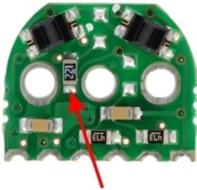
one current-limiting resistor (IR LEDs in series)
