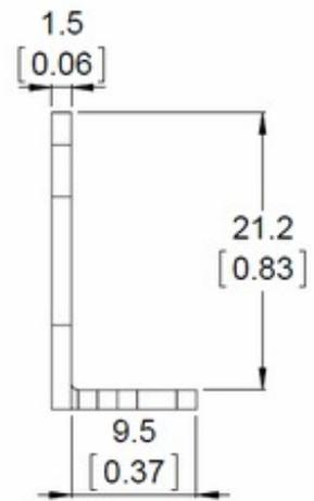
Mechanical drawing for the Pololu stamped aluminum L-bracket for plastic gearmotors. Units are mm over [inches].
