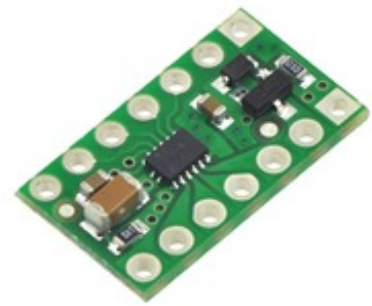
DRV8835 dual motor driver carrier.
