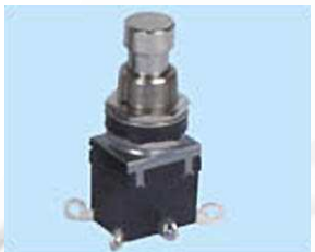
PS24202 ON-ON PS24212 ON-(ON) 4 A 125 VAC; 2 A 250 VAC DPDT 6P (L=14.2, 11.8, 9.8)
