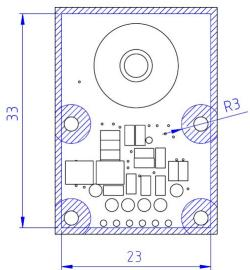
Only use hatched areas for mechanical assembly (screws, nuts, etc).
