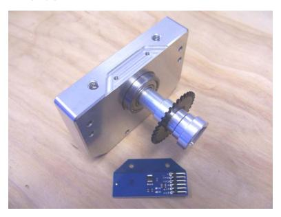
Step 2: Next insert the bearing and axle into the Motor Mount block. Be sure to fully-seat the bearing into the block as shown below.
