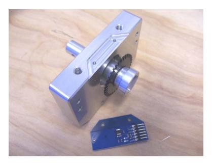
Step 3: Mount the Encoder board to the Motor Block, using the two flat-head screws provided. Be sure to align the board such that the Encoder disk fits between the slots of the encoder sensor on the PCB, as shown below.
