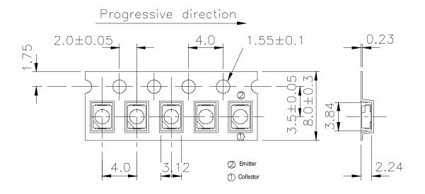
TOLERANCES UNLESS DIMENSION±0.1 ANGLE±0.5 UNIT:mm
