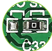
Figure 5-1: zero-ohm J1 jumper
