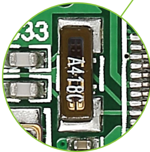
Figure 6-1: 32.768 kHz crystal oscillator module (X2)
