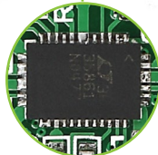
Figure 5-2: power management and battery charger IC
