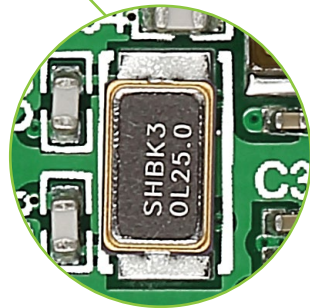
Figure 6-2: 25MHz crystal oscillator module (X1)
