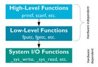
The high-level and low-level functions are not target-dependent and use the system I/O functions to interface with hardware.
