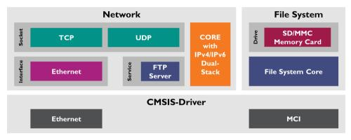
As explained before, CMSIS-Driver provides the interface between the microcontroller peripherals and the MDK Middleware.
