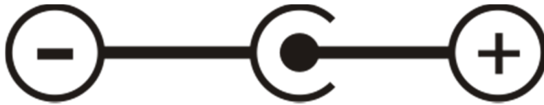
Figure 3 Barrel Connector J7 Polarity
