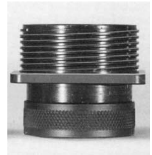
Standard double-lead Acme. Two parallel threads.
