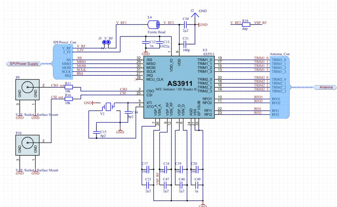
Figure 5: Filter and matching network
