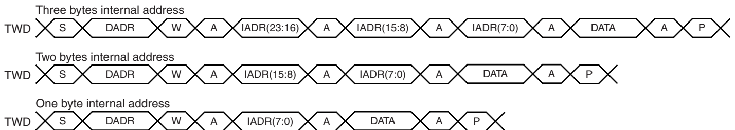
Figure 38-12. Master Write with One, Two or Three Bytes Internal Address and One Data Byte
