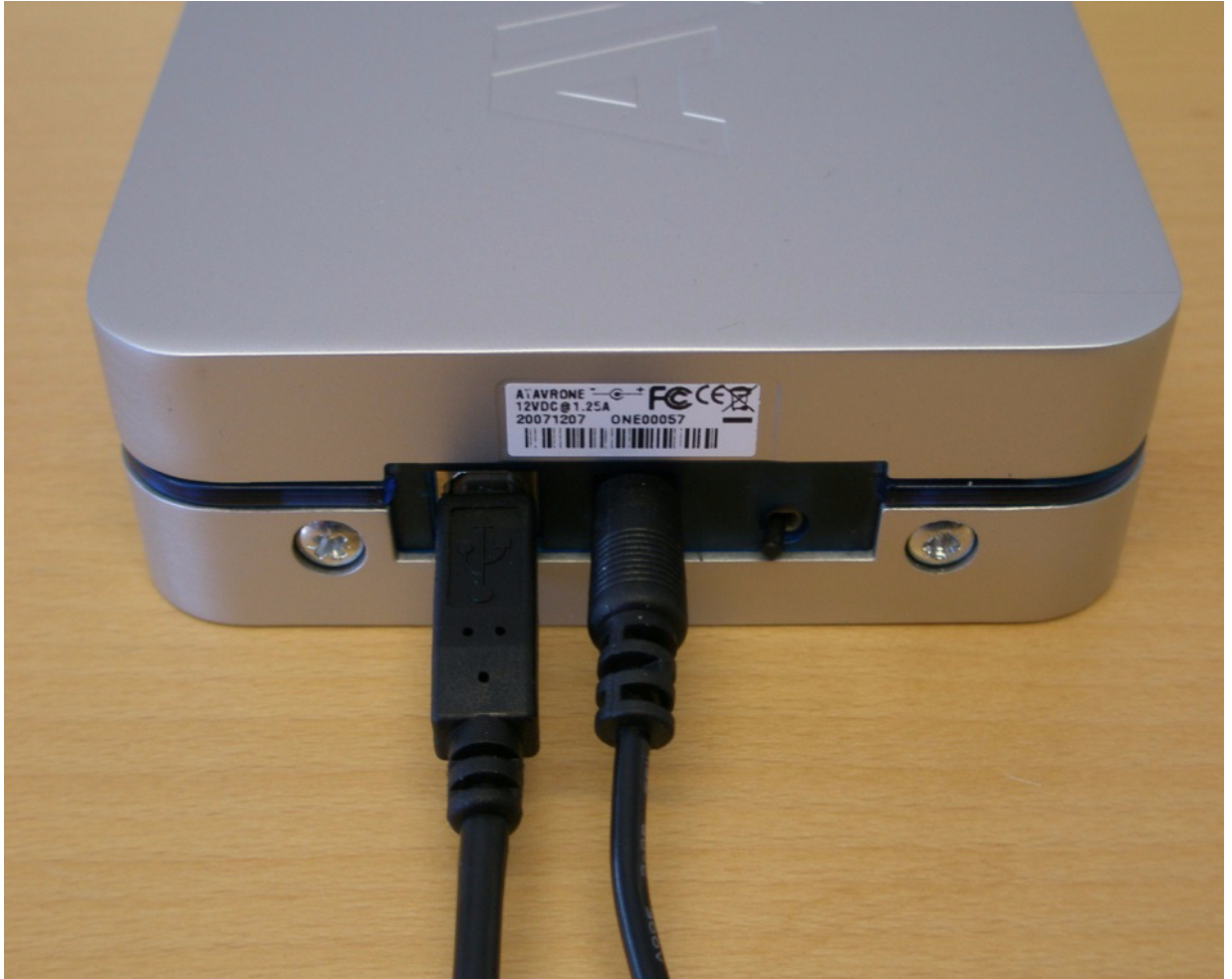
Figure 4-19. AVR ONE! connected to power and USB
