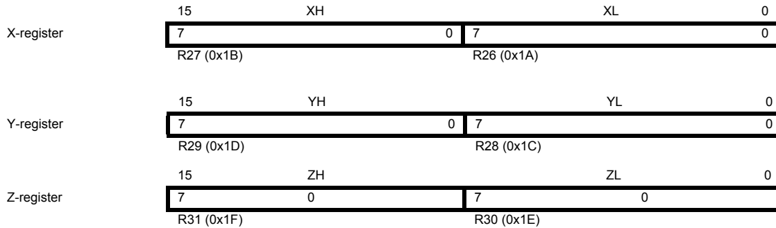
Figure 4-3. The X-, Y-, and Z-registers
