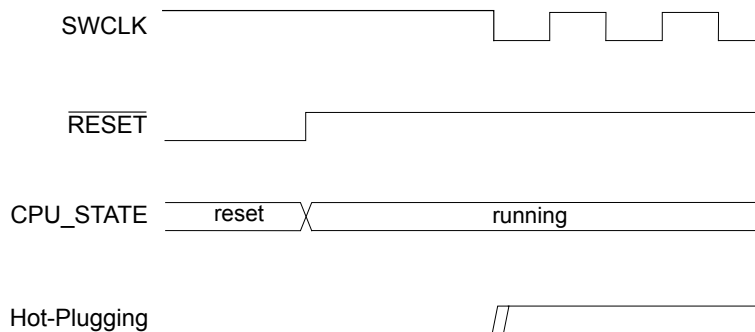
Figure 13-3. Hot-Plugging Detection Timing Diagram
