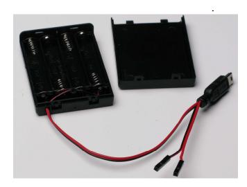
Power supplied via mini USB connector and battery pack connected to kit backside with "Velcro".
