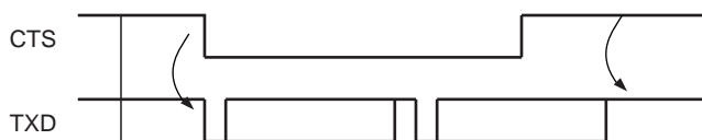
Figure 44-28. Transmitter Behavior when Operating with Hardware Handshaking
