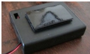
Glue Velcron to battery case
