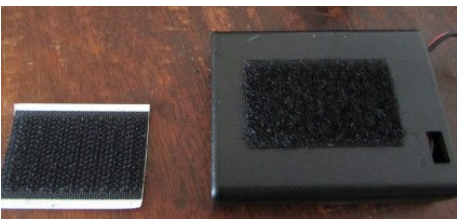
Glue Velcron to battery case
