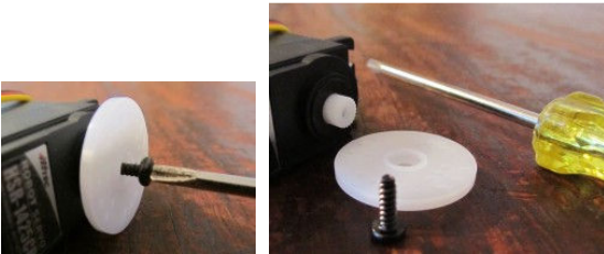
Remove the center screw
