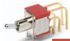
7201MD9AV2BE Vertical Actuation DPDT
