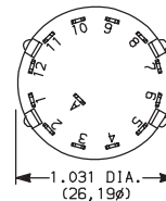
TERM. NOS. MOLDED ON HOUSING
