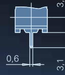
PCB terminal 1,3x0,5 mm straight
