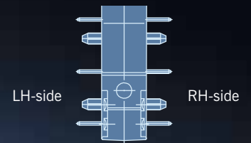
Side definition with terminals and location pins
