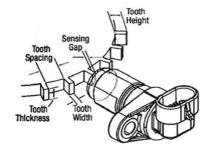
For best results, we recommend targets made from low carbon cold rolled steel. Other factors that influence sensor performance include gear tooth height and width, space between the teeth, shape of the teeth and thickness of the target. As a general guideline, consider a target with minimum parameters as shown below. Note that smaller dimensions may work, but testing for the application is required.
