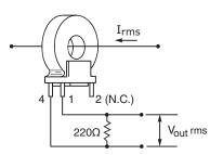
The CS60 series is designed to measure current from 5 to 100 Arms. Applications include sensing branch circuit overload and detecting load drop or shutdown. The sensor functions as the encapsulated secondary of a current transformer, while the conductor carrying the current to be measured serves as the "one turn primary." Sensitivity may be enhanced by increasing primary turns.
