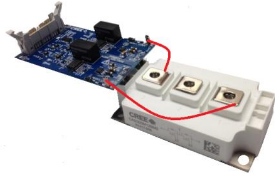
Figure 6. CGD15HB62P1 Mounted with Desat Connections
