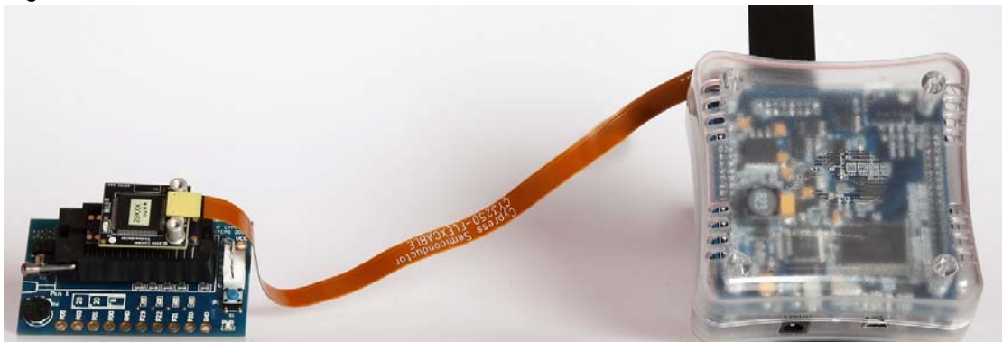
Figure 3-10. Flex Pod Connected to ICE-Cube Pod
