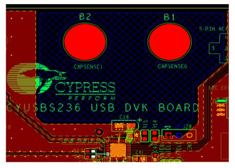
Figure A-9. CapSense Layout - Ground Layer
