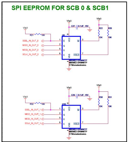
Figure 4-15. SPI Interface (SCB0 and SCB1)
