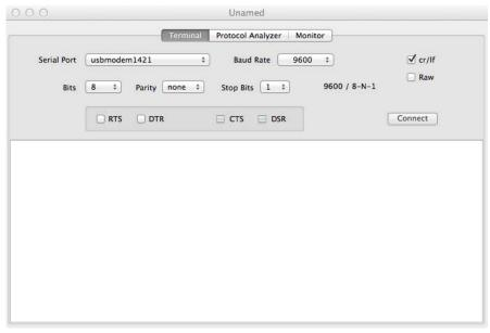
Figure 5-1. Connecting USB-Serial Device in Serial Tools
