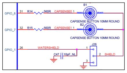
Figure 4-17. CapSense Schematic
