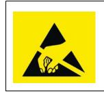
The CYUSBS236 kit contains electrostatic discharge (ESD) sensitive devices. Electrostatic charges readily accumulate on the human body and any equipment, and can discharge without detection. Permanent damage may occur on devices subjected to high-energy discharges. Proper ESD precautions are recommended to avoid performance degradation or loss of functionality. Store unused CYUSBS236 boards in the protective shipping package.
