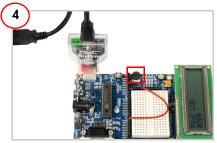
Open PSoC Programmer; click on the Toggle Power button to power the board.
