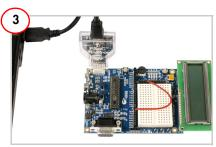
Plug in the MiniProg to the ISSP header on the CY3210-PSoCEVALL board.
