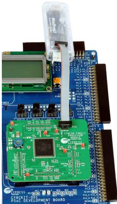
Figure 2-16. Connect MiniProg3 to J5 on CY8C38 Family Processor Module
