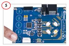
Touch the CapSense button CSB5 to change the HBLED brightness. There are 10 brightness levels for each HBLED.
