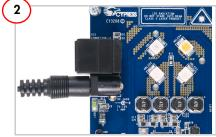
Plug in the power supply. LED1 (green) turns ON.
