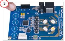
Touch the CapSense buttons CSB1 to CSB4 to turn on the HBLEDs. Touch them again to select corresponding HBLED.
