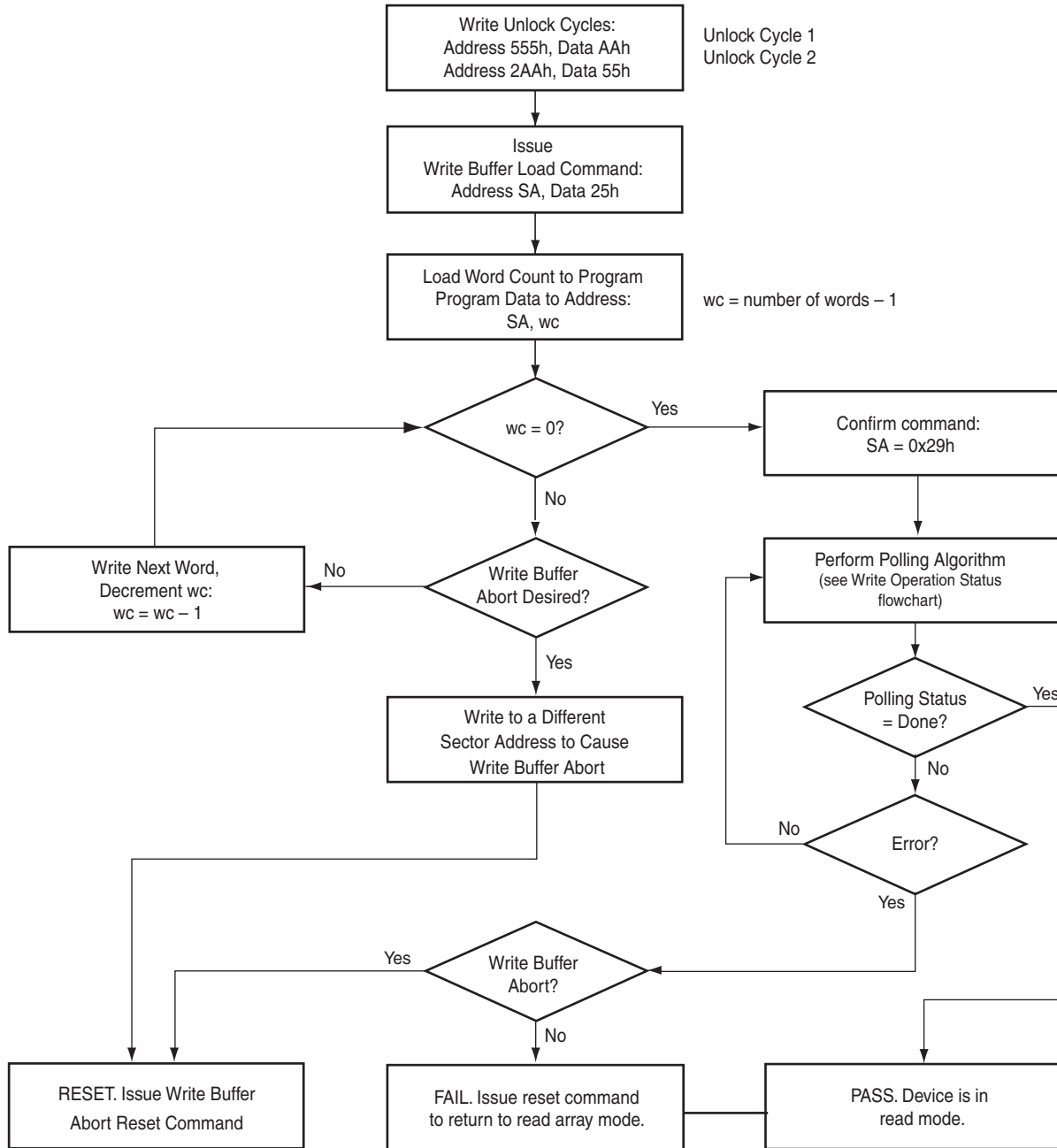
Figure 7.2 Write Buffer Programming Operation
