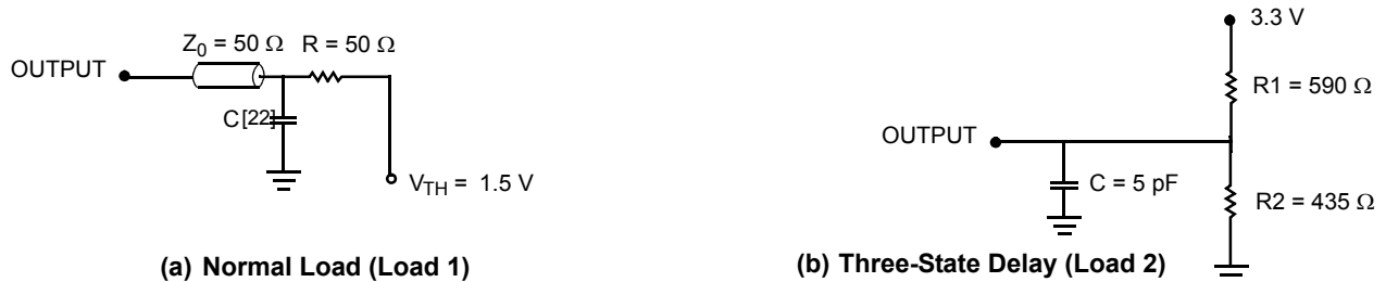
Figure 3. AC Test Loads and Waveforms
