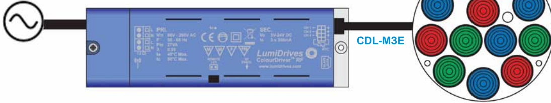
Typical Connection - With Color Engine 12
