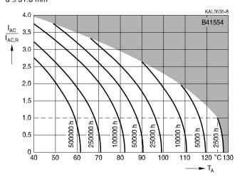
**Useful life** $^{1)}$  depending on ambient temperature  $T_A$  under ripple current operating conditions  $d \ge 64.3 \text{ mm}$
