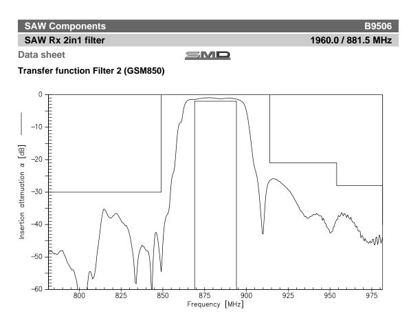
Transfer function Filter 2 (GSM850) - Wideband
