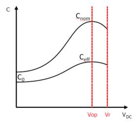
Initial capacitance C<sub>0</sub>: Is the value at the origin of the hysteresis without any applied direct voltage.
