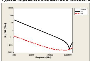
$V_{DC} = 0 \text{ V}, V_{AC} = 0.5 \text{ V}_{RMS}, T_{device} = 25 \text{ °C}$
