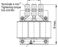
PE M4 / Tightening torque 1.2±0.1 Nm
