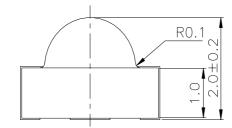
For reflow soldering (propose)
