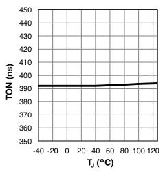
Figure 10:  $T_{ON}$  versus temperature,  $R_{ON}\text{=}16.2k\Omega$
