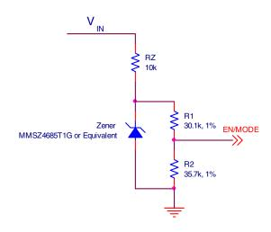
Figure 25: Selecting Forced CCM by deriving EN/MODE from  $V_{\rm IN}$
