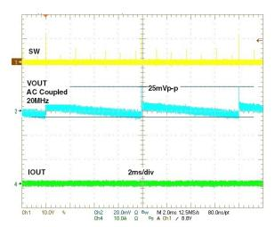
Figure 14: Steady state, DCM, I<sub>OUT</sub>=0A
