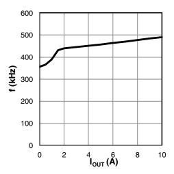
Figure 5: frequency versus I<sub>OUT</sub>
