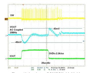
Figure 18: Load step, DCM/CCM, 0A-5A-0A
