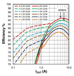
Figure 21: Efficiency, V<sub>IN</sub>=12V
