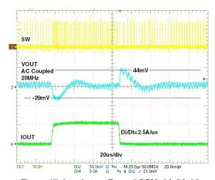
Figure 17: Load step, Forced CCM, 0A-5A-0A
