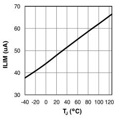
Figure 9: I<sub>LIM</sub> versus temperature
