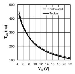
Figure 4: T<sub>ON</sub> versus V<sub>IN</sub>, R<sub>ON</sub>=6.98k
