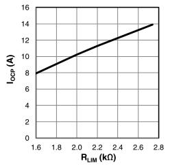
Figure 7: I<sub>OCP</sub> versus R<sub>LIM</sub>
