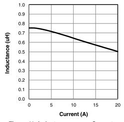
Figure 11: Inductance versus Current
