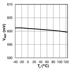
Figure 8: V<sub>REF</sub> versus temperature
