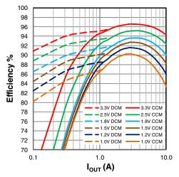
Figure 19: Efficiency, V<sub>IN</sub>=5V
