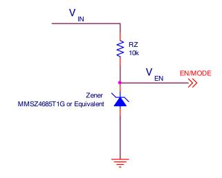
Figure 26: Selecting DCM/CCM by deriving EN/MODE from  $V_{\rm IN}$
