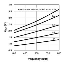
Figure 12:  $V_{OUT}$  versus f,  $V_{IN}$ =12V
