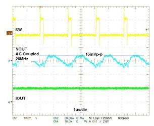
Figure 13: Steady state, CCM,  $I_{OUT}$ =10A
