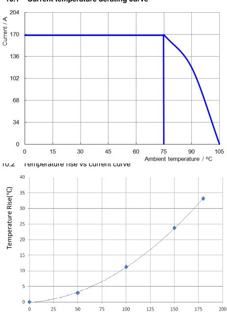
Above rating is for reference only. Appropriate de-rating is required per ambient conditions, bus bar size to achieve thermal balance, gross heating from adjacent components, and other factors that influence connector performance.
